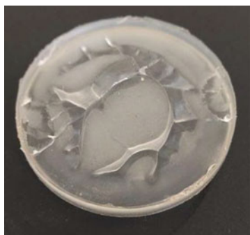
Fig. 6 Moulds formed of fractals using PDMS
