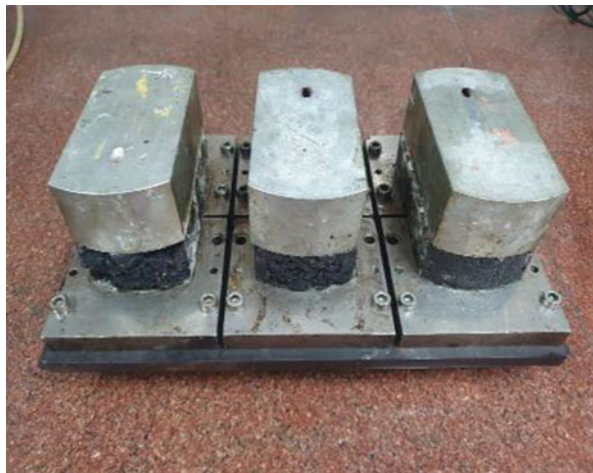
Fig. 2 Trimmed specimen glued to plate
