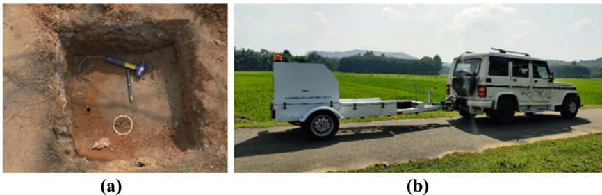
Fig. 1 Photos illustrating a Test pit and b FWD equipment
