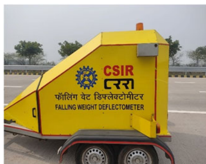
Falling Weight Deflectometer (FWD)
