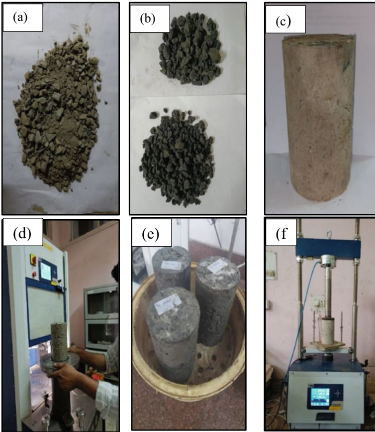
Fig. 3 a Aggregate used in specimen preparation, b Single-sized RAP material used, c Gyratory compaction of specimens, d Compacted UCS specimen, e Curing of specimens in the desiccator, f Unconfined compressive strength test in the laboratory
