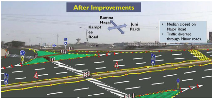
Fig. 6 Typical illustration of Chikli square option 2 having junction closure on the major approach
