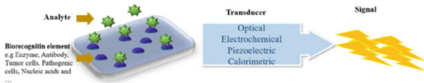
Fig. 6.1 Schematic representation of a biosensor. (Reproduced with permission from (Ameri et al. 2020))
