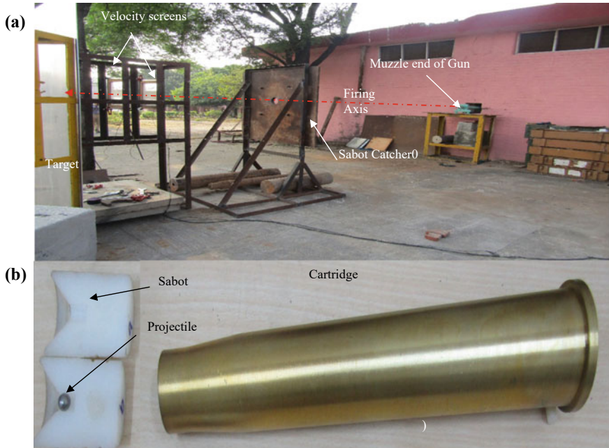
Fig. 1 a Test setup, b projectile, sabot and cartridge
