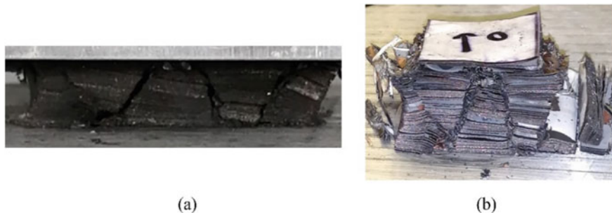
Fig. 4 Failure modes of jellyroll in the compression tests a Constant speed mode; and b Impact mode
