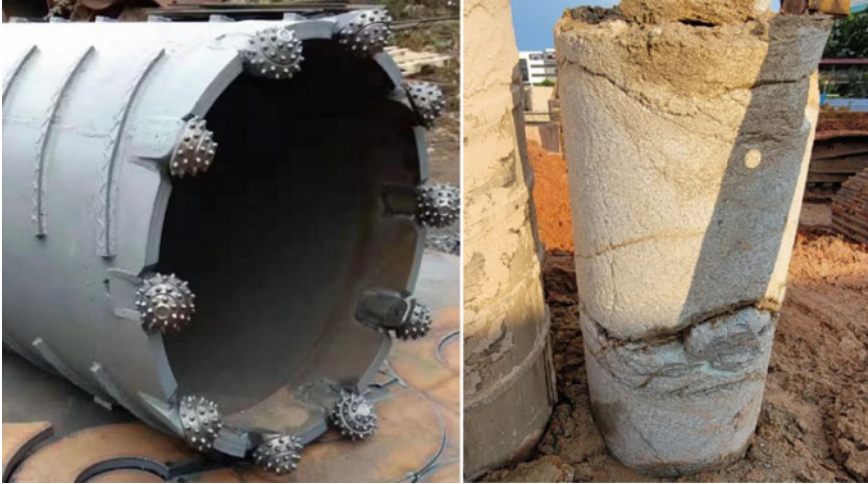
Fig. 1 Core barrel-roller bit and rock core sample by using core barrel-roller bit
