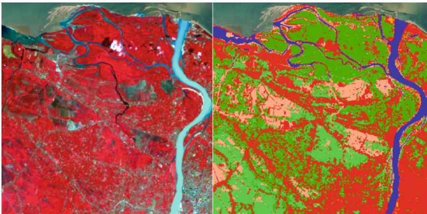
Fig. 5 Part of original Landsat-8 image with false color composite at left, and the same part in the classified land cover map at right for comparison. The legends of classes are same as in Fig. 7
