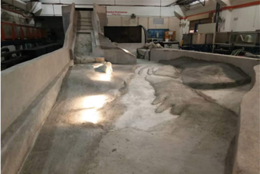
Fig. 2 Physical model of Kenyir Dam spillway
