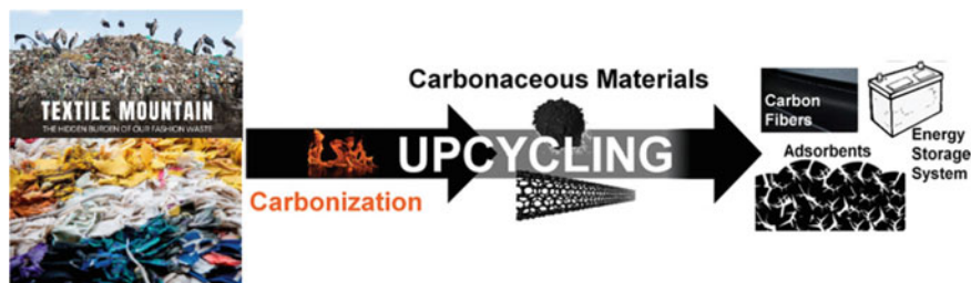
Fig. 10.1 Upcycling of fibrous wastes to carbon-based functional materials (Choi et al. 2022)
