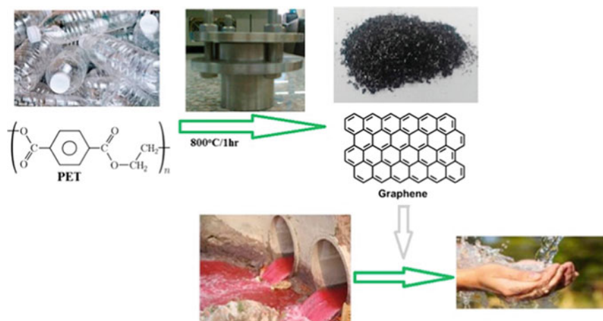
Fig. 10.10 Active carbon from single-use solid plastic waste (El Essawy 2017a)
