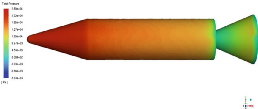
Fig. 8 Total pressure variation on the rocket motor
