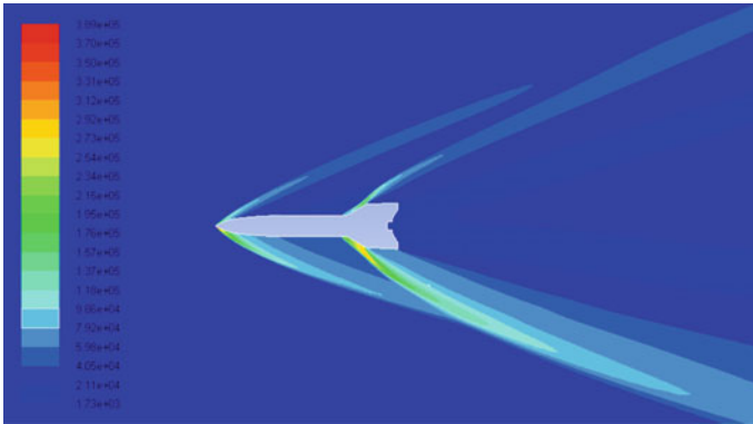
Fig. 7 Contour of pressure at M = 4.5 and AoA = 5^\circ
