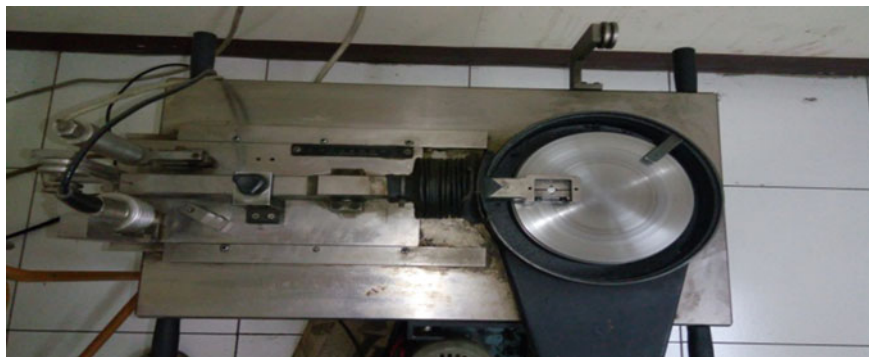
Fig. 2 Pin-on disc wear testing machine
