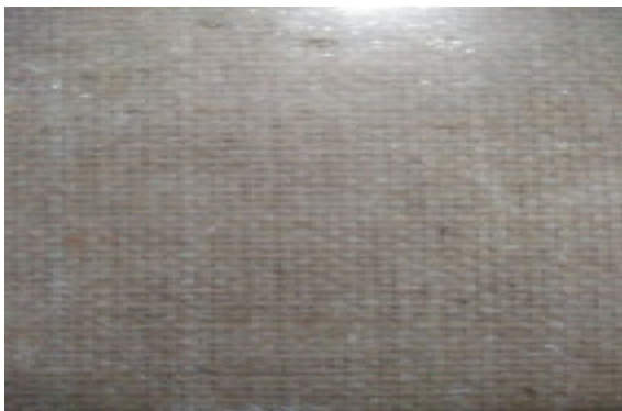
Fig. 1 Fabricated composite plate-Plate 1 (Sisal-Jute-Sisal)
