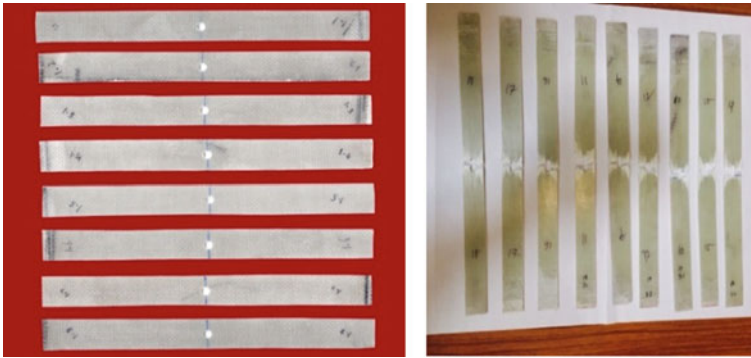
Fig. 5 Open hole tensile and fractured tensile specimens
