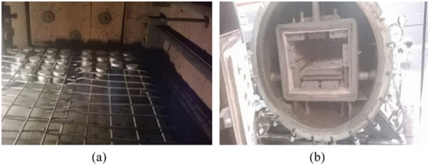
Fig. 7 Sintering process a samples kept inside the furnace and b outer view of the furnace
