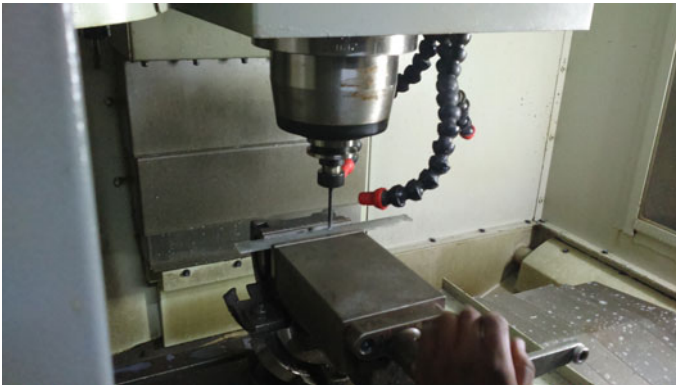
Fig. 2 Drilling experimental setup
