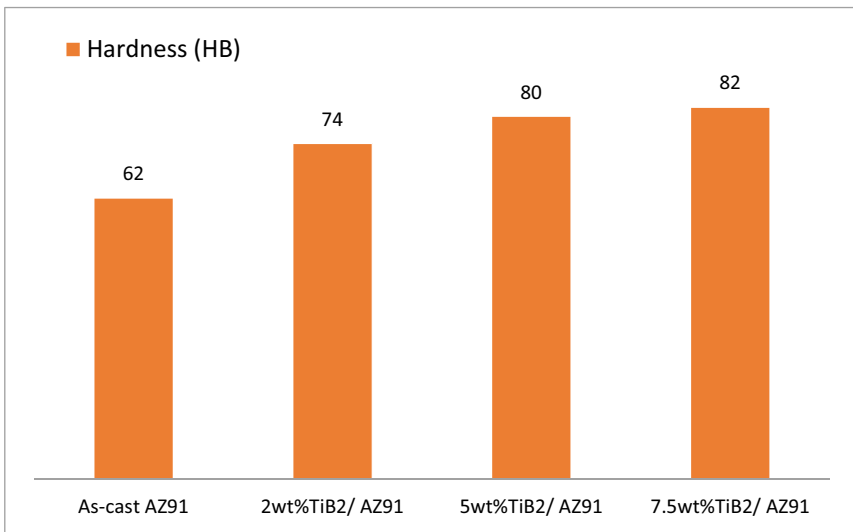
Fig. 1 Brinell hardness values of Mg composites strengthened with TiB 2
