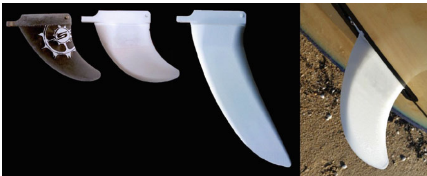
Fig. 11 Comparison of the 2016 G-Whiz Slingshot SUP's original centre fin with versions made similarly using desktop FFF (second), and selective laser sintering (third) (3rd). One of the fins installed on the SUP board is shown in the right image [54]
