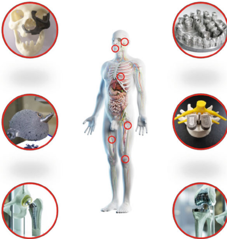
Fig. 3 The schematic depiction of the biomedical application of additive manufacturing of biomaterials includes the cranial prosthesis, dental implants, acetabular cup, interbody fusion cage, hip prosthesis, and knee prosthesis [25]
