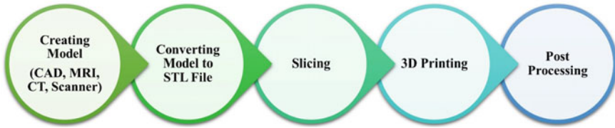
Fig. 2 Steps of additive manufacturing process
