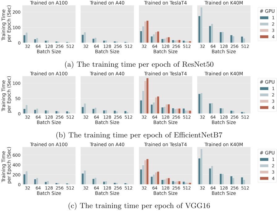
Fig. 2. The training time of DL models for specific batch size on several GPU architectures
