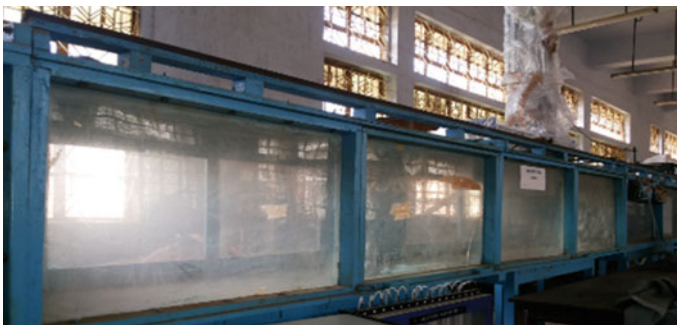
Fig. 1 Photograph of wind tunnel and model in the open-circuit wind tunnel
