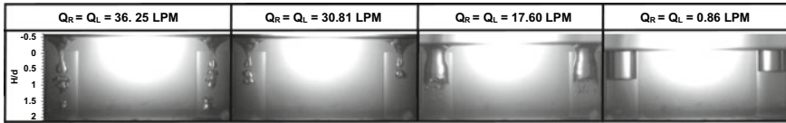
Fig. 5 Obtained possible symmetry fluidic structures at P = 5d for the different average liquid discharge rates
