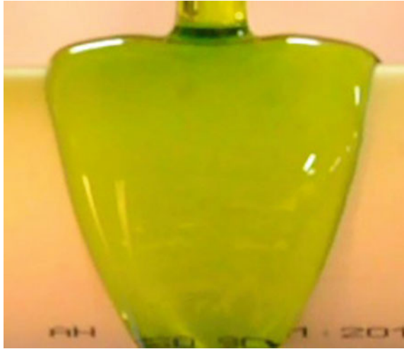
Fig. 3 Original image of the fluid flow over horizontal cylinder used for wetting area calculation
