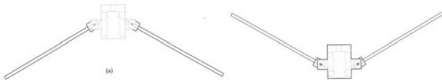
Fig. 1 Extreme location of the fins a at the end of downstroke b at the end of the upstroke
