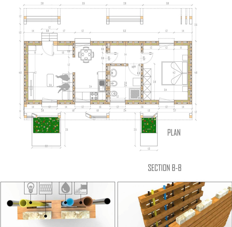
Fig. 6. Design of the local building organism. Case study with residential use: plan, and detail of facilities and insulation of the pallet module.
