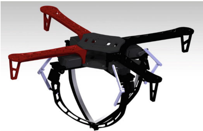
Fig. 11 Retracted landing gear CAD model
