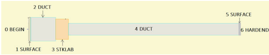
Fig. 9 Schematic view of the resonator as per Amirin et al. [13]
