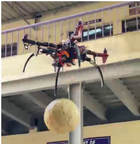
Fig. 22 A distinct perspective of the quadcopter as it drops the payload by retracting its landing gears outwards
