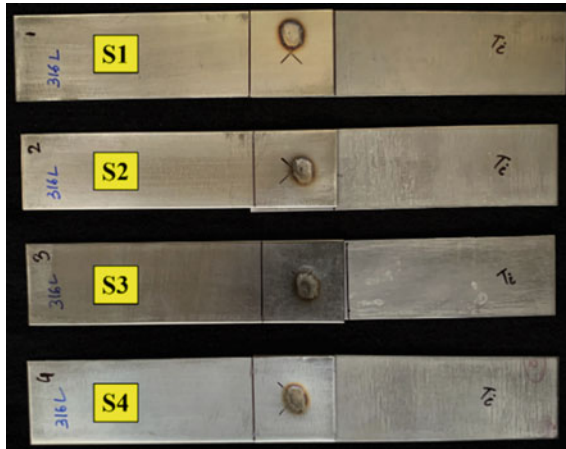
Fig. 3 RSW joints fabricated at different process parameters (S1, S2, S3, and S4)
