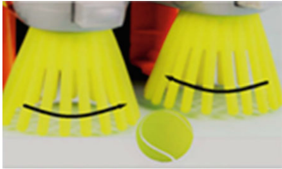
Fig. 5 Collecting using two cylinders with vertical actuator
