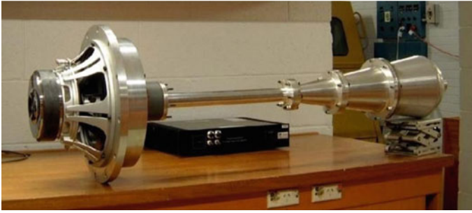
Fig. 1 Model of a thermoacoustic refrigerator [1]
