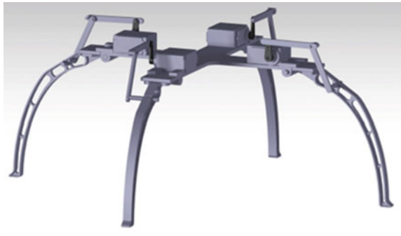
Fig. 15 Isometric view of X-Type hinge and rotating hinge
