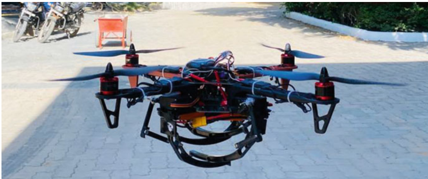
Fig. 19 Quadcopter with fully retracted landing gears in air without payload
