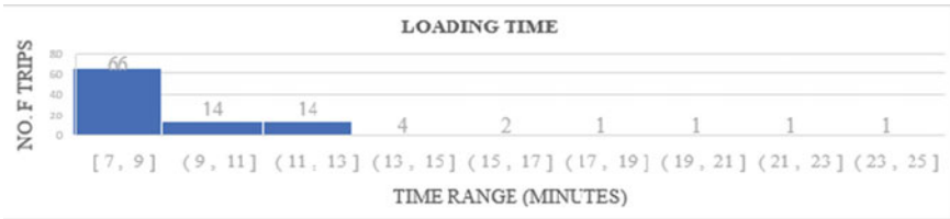
Fig. 7 Histogram for loading time of Transit mixers
