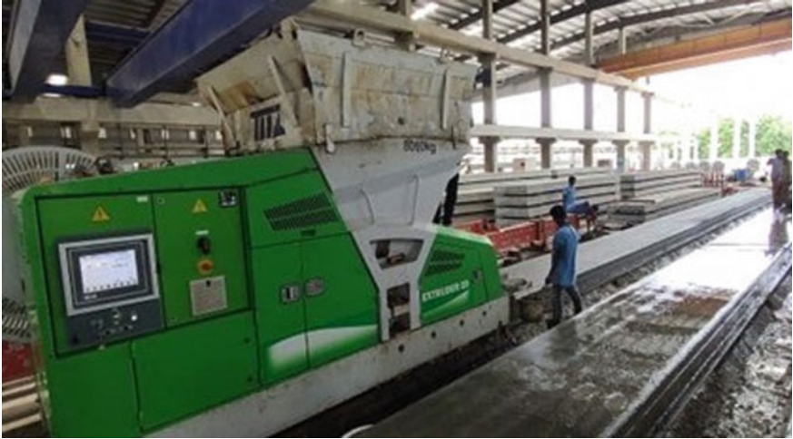
Fig. 2 Hollow-core slab extruder machine
