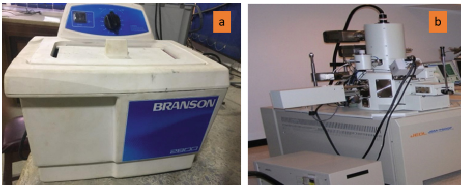
Fig. 2. Equipment for Nanofluid preparation (a) Ultrasonic Bath. (b) JEOL-JSM 7600F Scanning Electron Microscope.
