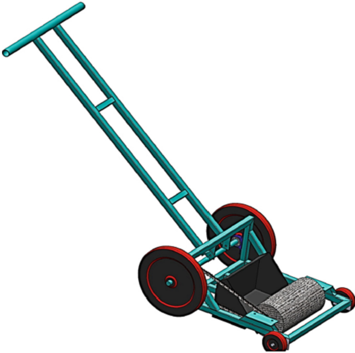
Fig. 1. CAD assembly of a hand operated sweeping machine.
