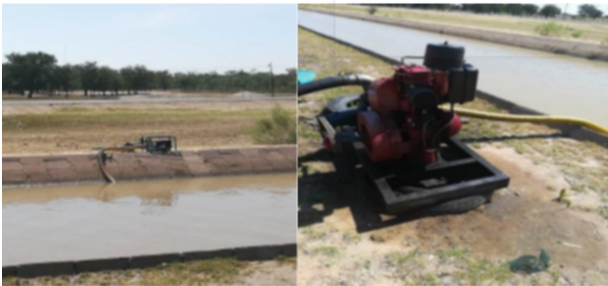
Fig. 1. Diesel water pump used by the small-scale farmers.
