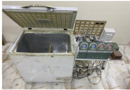
Fig. 2. The evaporator tube loop and the insulation cover.
