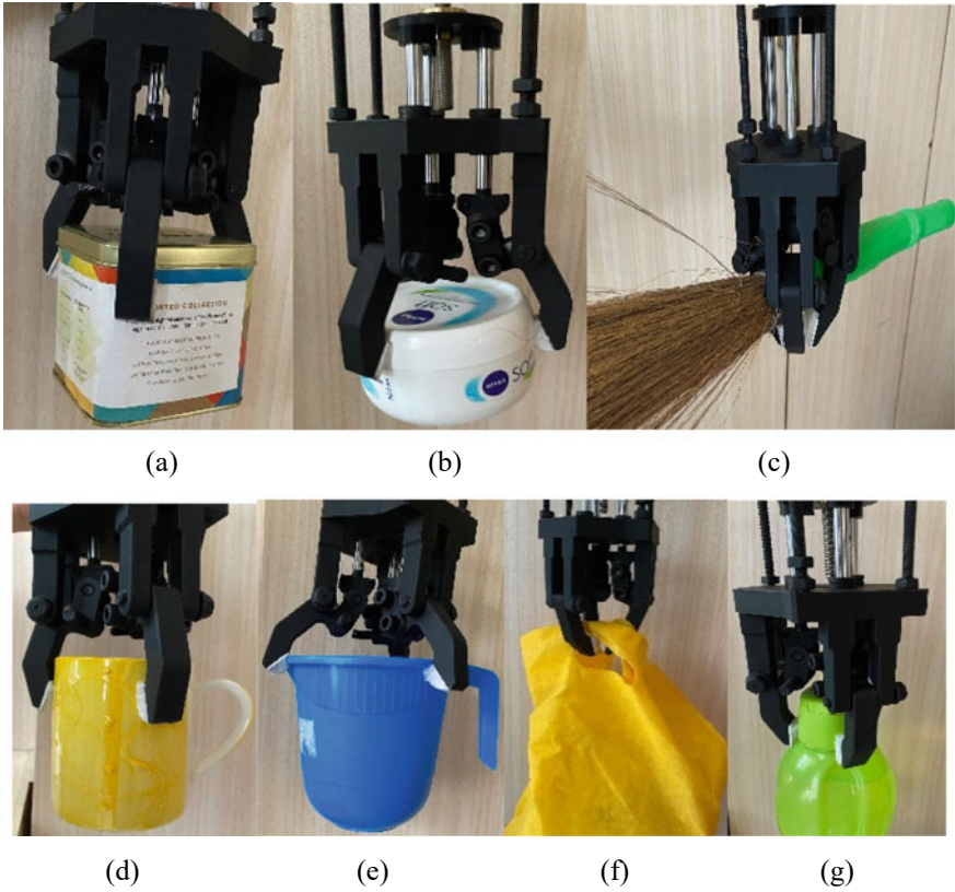
Fig. 6.6 Examples of grasps: a square box; b cylindrical object; c broom; d cup; e mug; f bag; g bottle
