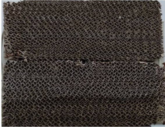
Fig. 9.6 Honeycomb pads for lowering down the power consumption of compressor
