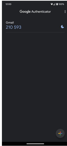
Fig. 1. Screenshot (Screenshots are taken from the Android SDK emulator, because the OS prevents screenshots since the app is flagged as secure.) of the Google Authenticator app showing a TOTP code generated for account authentication.
