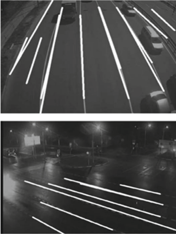
Fig. 2 Road marking detection
