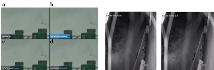
Fig. 8 a Original scaled 50%, b Theia fine tune fidelity: 4K rendering, c Theia fine tune fidelity: 4K not rendered, d Artemis high quality: 4K not rendered, zoomed at 36%. Theia fine tune fidelity: 4K rendering is found to be best compared with Artemis high quality: 4K not rendered. The objects in Fig. 8b are seen with clear edges than in the output of Artemis high quality model
