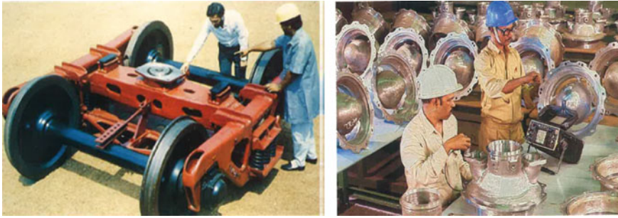
Fig. 3.2 CASNUB bogie developed for the Indian Railways and alloys steel castings of Kurla foundry
