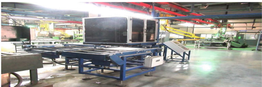
Fig. 17.10 Automatic pellet stacking machine
