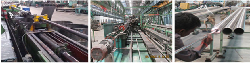
Fig. 17.22 Grinding & honing operations in PT production
