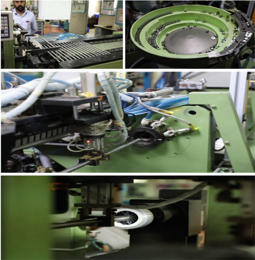
Fig. 17.14 Integrated end cap welding and machining unit. a Tube machining, b End cap feeding, c End cap welding, d Element machining
