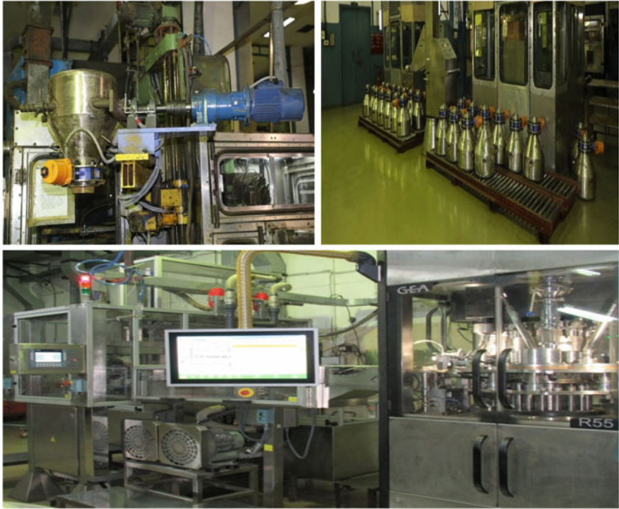
Fig. 17.9 a Integrated blending & granule transfer system. b Rotary compaction press
