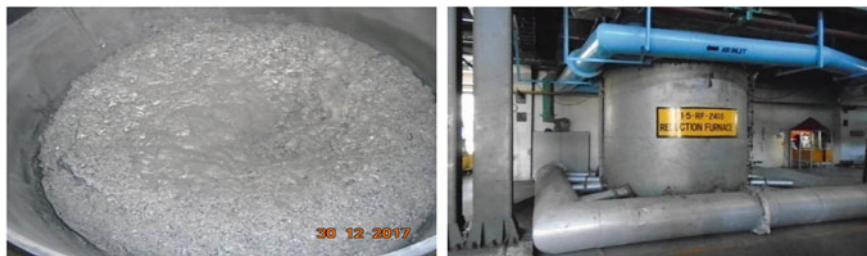
Fig. 17.21 1500kg Zr-metal produced and Facility for its production
