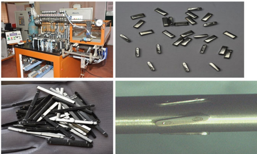
Fig. 17.13 Integrated spacer & bearing pad welding unit
