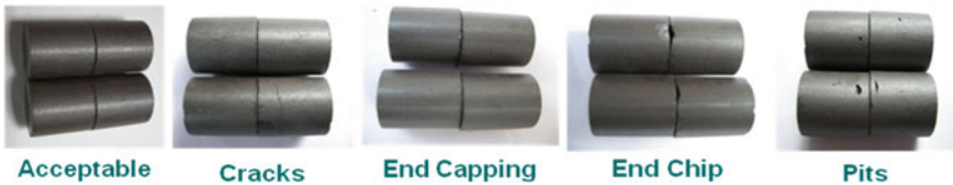
Fig. 17.19 Automated visual inspection of UO2 pellets
