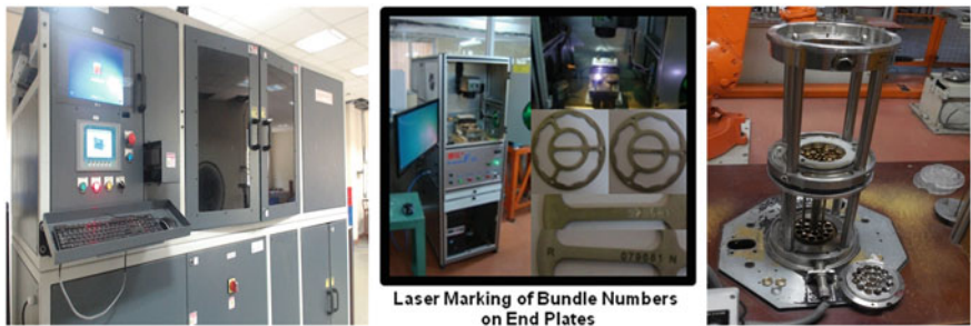
Fig. 17.20 a Vision-based tube inspection system, b Laser marking of bundle numbers on end plates, c Metallic Jig for PHWR bundle fabrication
