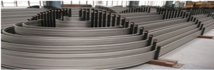
Fig. 17.25 Incoloy-800 U bend SG tubes
