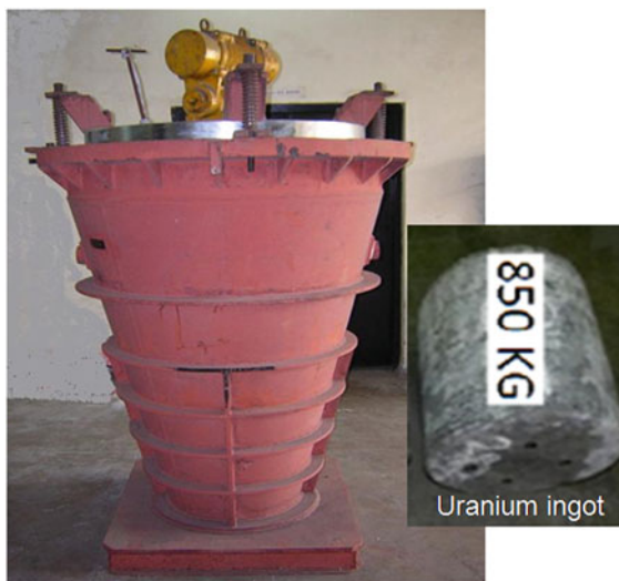
Fig. 12.3 Reactor used for metallothermic reduction of UF 4 for making uranium metal (inset: U metal ingot)
