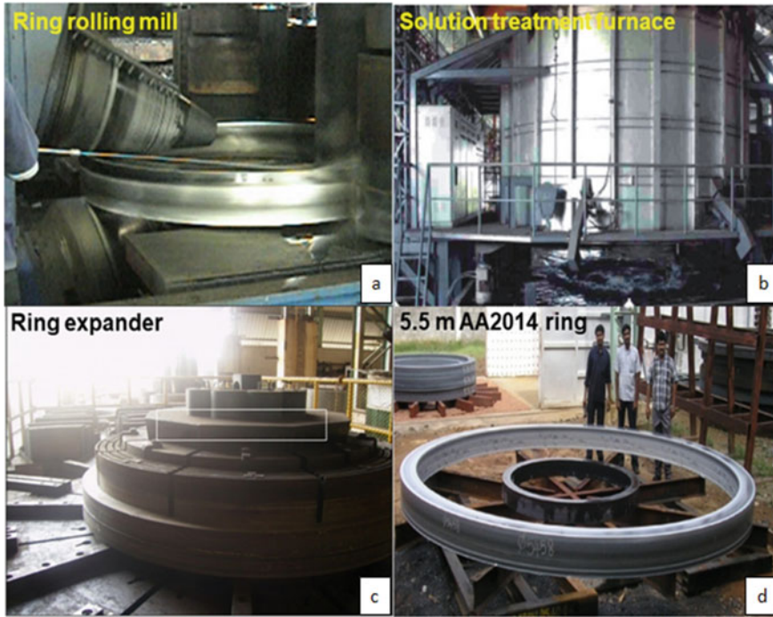
Fig. 16.4 Processing of large diameter aluminium alloy rolled rings essential for the fabrication of propellant tanks and inter tank structures of launch vehicles. The figure shows the a ring rolling mill under operation, b solution treatment furnace with drop bottom quenching facility, c ring expander to impart the desired temper and d a large size rolled ring
