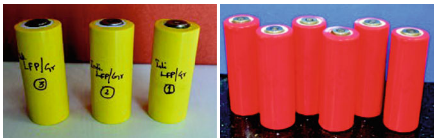
Fig. 20.25 LFP/graphite cells and NMC/LTO cells with indigenously developed LFP and LTO powders
