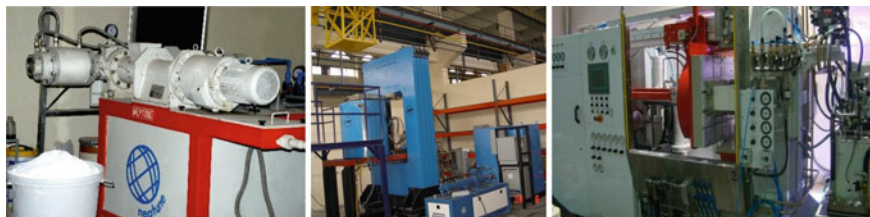
Fig. 20.15 (left) Screw type extruder for extrusion of high symmetric ceramic parts, (centre) hot isostatic press, (right) pressure slip casting machine
