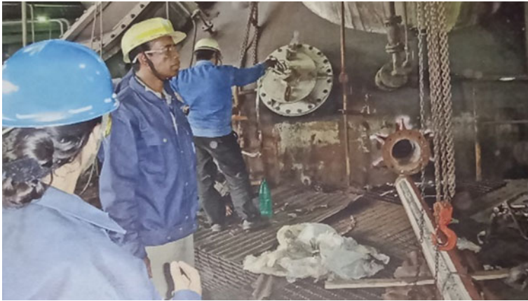
Fig. 1.8 Probing the blast furnace using an advanced material trajectory probe (2010)
