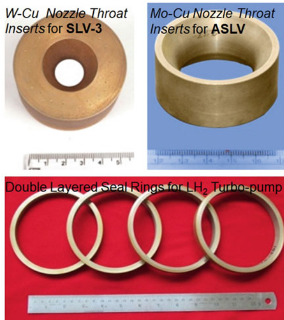
Fig. 16.9 Powder metallurgical products used in satellite launch vehicles. These include W-Cu nozzle throat inserts for SLV-3, Mo-Cu nozzle throat inserts for ASLV and double layered bronze seal rings for LH 2 turbo-pumps of C25 engine of GSLV MkIII
