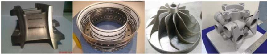
Fig. 20.19 (left to right) Laser drilled HP NGV, aero-engine Combustion liner, laser drilled HP NGV, and additively manufactured gas manifold block
