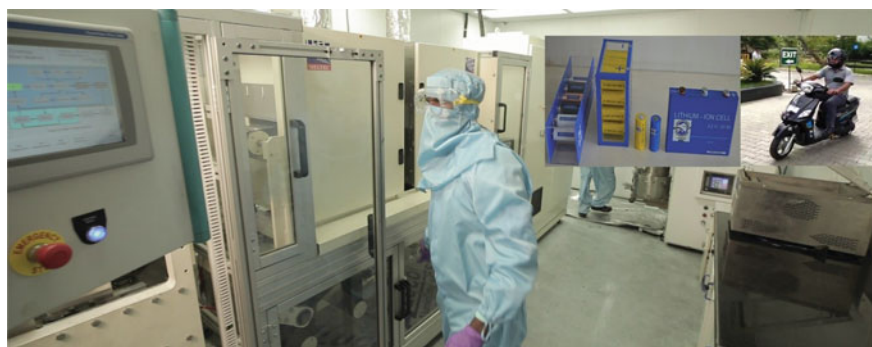
Fig. 20.24 Li-ion battery fabrication facility. Insets show batteries fabricated at ARCI and e-scooter with Li-ion battery module developed at ARCI
