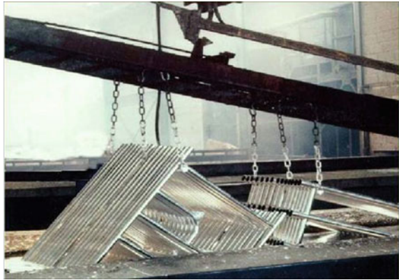
Fig. 13.3 A factory controlled metallurgical reaction of zinc and steel that provides “barrier” and “sacrificial protection” from corrosion
