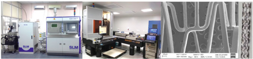
Fig. 20.20 (left) Additive manufacturing facility, (centre) ultra-fast laser machining facility, (right) cardiovascular stent sample micromachined and electropolished at ARCI
