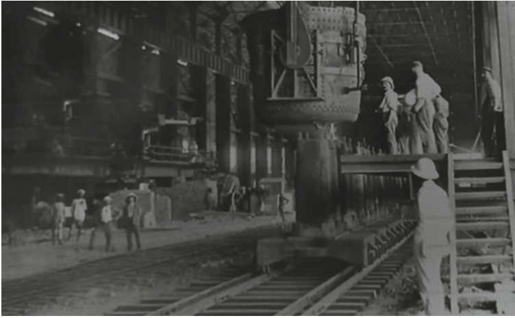
Fig. 1.9 First ingot casting steel from ladle into ingot mould (2 December 1911)
