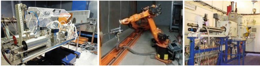
Fig. 20.12 (left) Advanced detonation spray system, (centre) cold spray coating system, (right) EB-PVD facility
