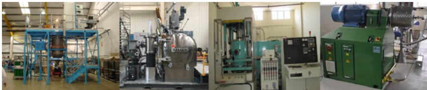
Fig. 20.5 Inert gas atomizer, induction melting furnace, inert gas atomizer, spark plasma sintering facility and Zox Simoloyer high energy milling
