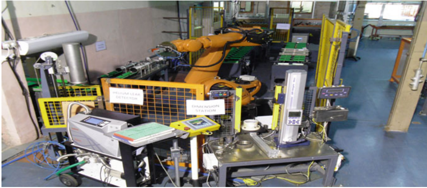
Fig. 17.18 Automatic fuel bundle inspection system
