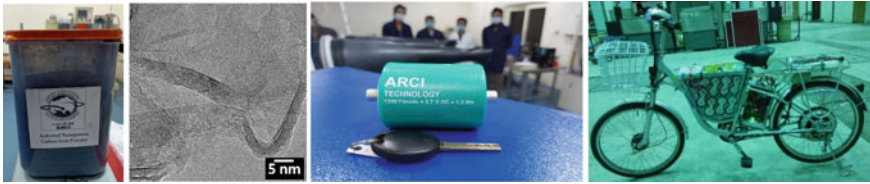
Fig. 20.11 (left) Petcoke derived porous Carbon powder and TEM image showing the presence of Graphene like structure, (centre) Indigenous Supercapacitor Device, (right) Demonstration of e-bicycle using indigenous supercapacitors
