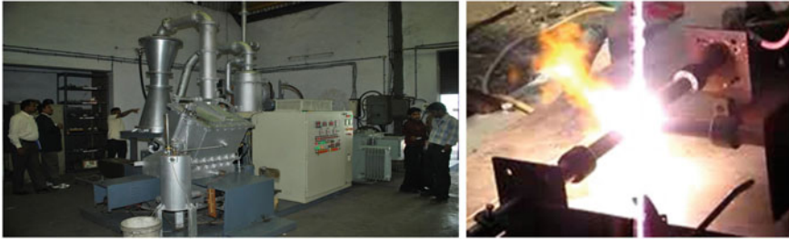
Fig. 19.2 Thermal plasma pyrolysis System and the plasma torch used for disposal of biomedical waste
