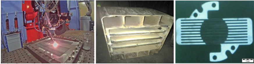
Fig. 20.18 Laser-coated baffle plate and its assembly in burner-tip nozzle of 200 MW thermal power plant, (right) laser cut micro-heater
