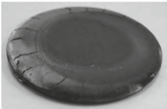
Fig. 12.4 Neodymium metal ingot produced by calcio-thermic reduction of its fluoride ( \text{NdF}_3 )
