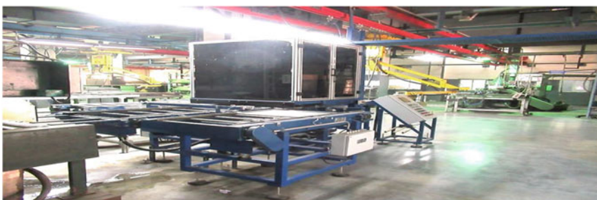
Fig. 17.10 Automatic pellet stacking machine
