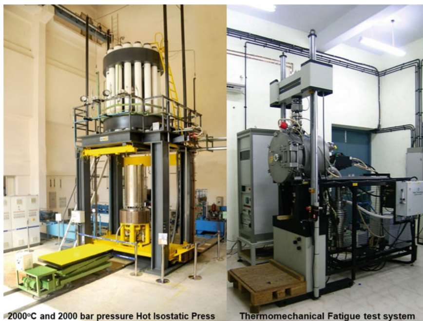
Fig. 16.11 State-of-the art facilities established in VSSC for processing and testing of materials
