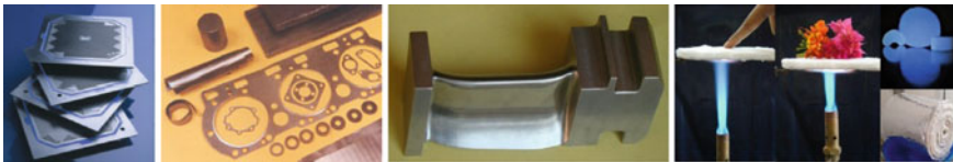
Fig. 20.4 (left) Exfoliated graphite products for various applications, (centre) Oxide dispersion strengthened steels for high-temperature applications, (right) Silica aerogel based thermal insulation sheets for oil and gas industries
