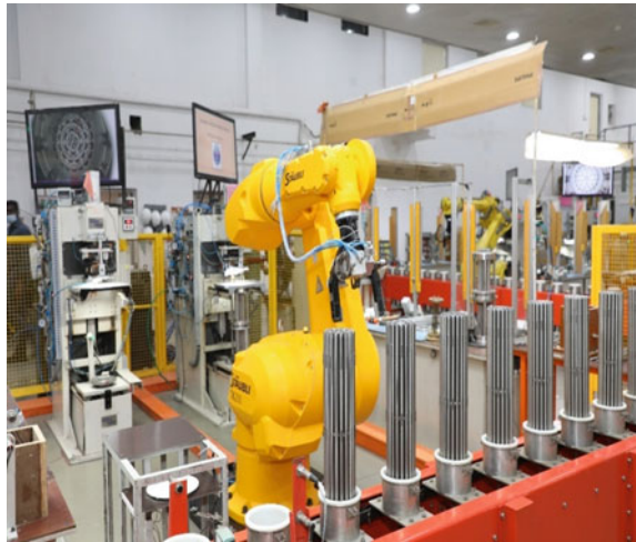
Fig. 17.15 Robotic end plate welding machine for 37 element PHWR fuel bundle
