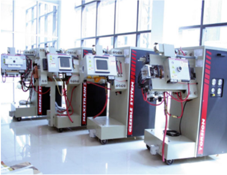
Fig. 1.12 Gleeble simulator for advanced thermomechanical simulation
