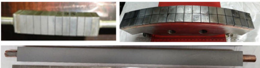
Fig. 19.5 a (top left) Tungsten mono-block divertor target test mock-up (Area: 100 \times 30 \text{ mm}^2 ), b (top right) Tungsten macro-brush dome test mock-up (Area: 350 \times 46 \text{ mm}^2 ), c (bottom) Tungsten coated test mock-up with CuCrZr substrate (Area: 440 \times 30 \text{ mm}^2 )
