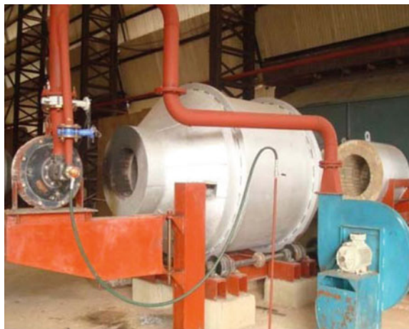
Fig. 14.2 Rotary furnace for Lead smelting
