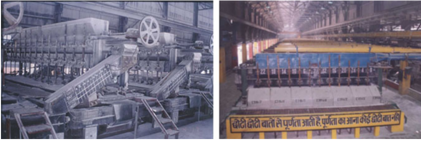
Fig. 6.2 Renukoot smelter plant before and after modernization-Covered pots with auto feeding
