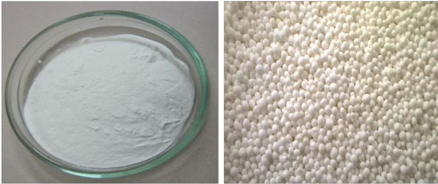
Fig. 19.3 \text{Li}_2\text{TiO}_3 powder and pebbles prepared at IPR
