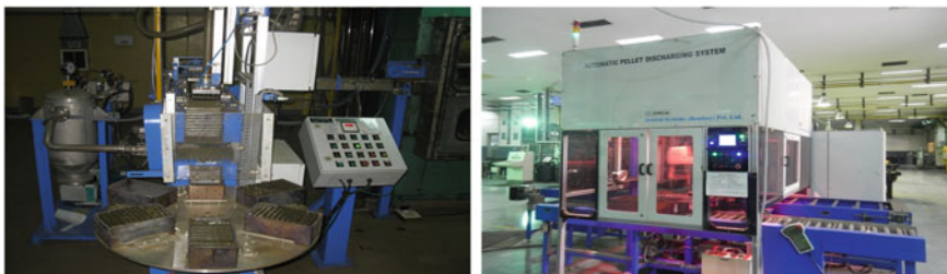
Fig. 17.12 a Automated Green Pellet charging system. b Sintered Pellet discharging system
