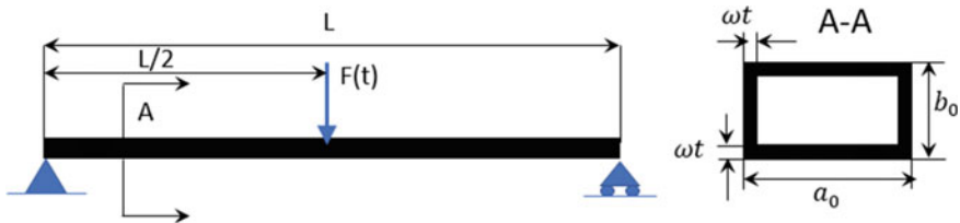
Fig. 3 Schematic diagram of the corroded beam
