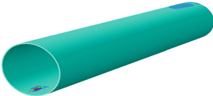
Fig. 12 Stress distribution ahead of crack tip
