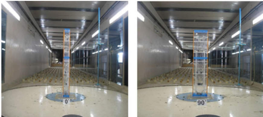
Fig. 2 View of the model of tall building in wind tunnel for a \theta = 0^\circ and b \theta = 90^\circ
