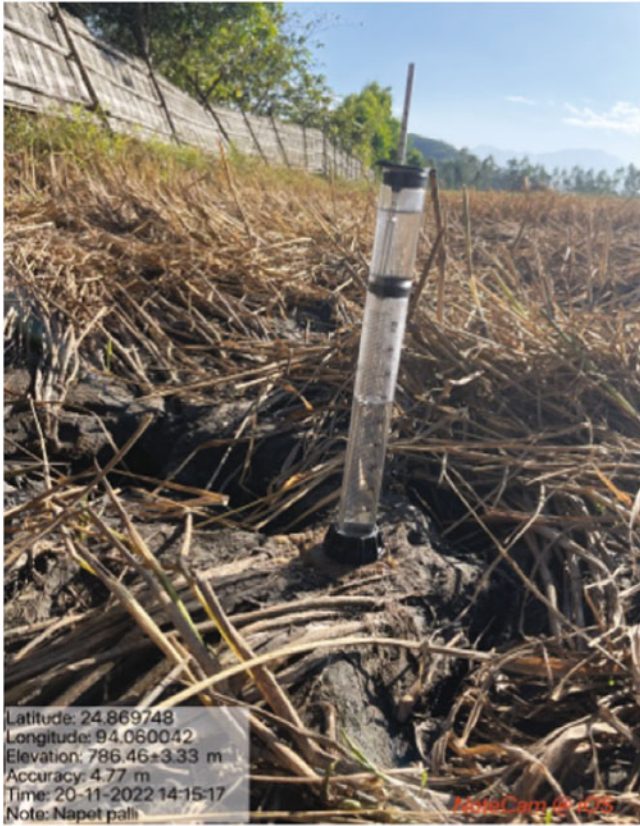
Fig. 3.3 Measurement of hydraulic conductivity using MDI at site
