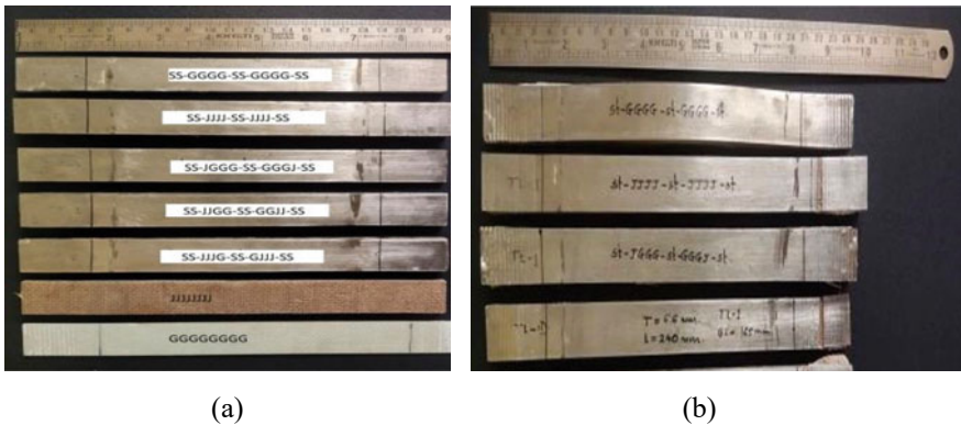
Fig. 3 a Tensile test specimens, b FML specimen failure after tensile test
