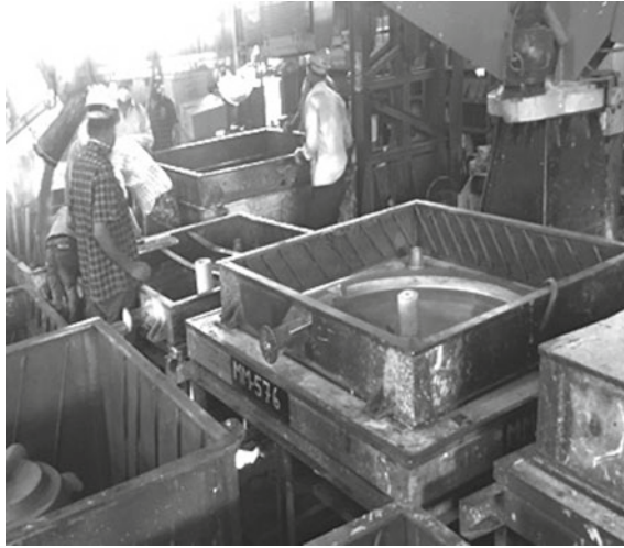
Fig. 7 Mold box preparation
