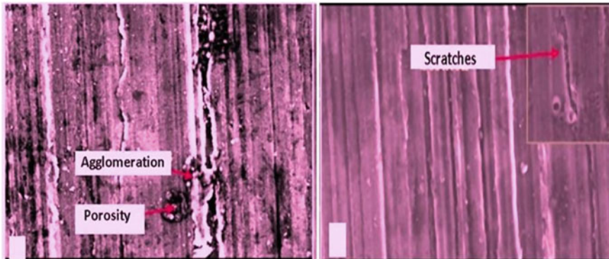
Fig. 3 Worn out surfaces of CNT-reinforced Mg alloy composite [47]
