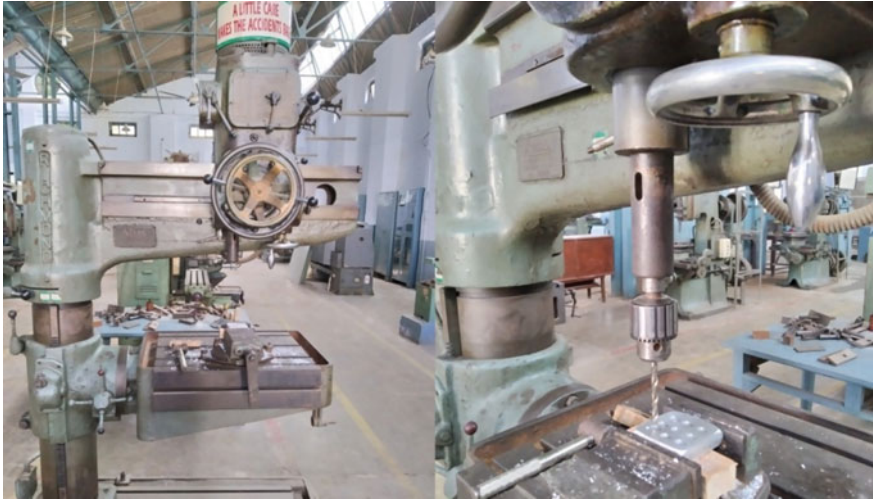
Fig. 1 Radial drilling machine and machined work piece
