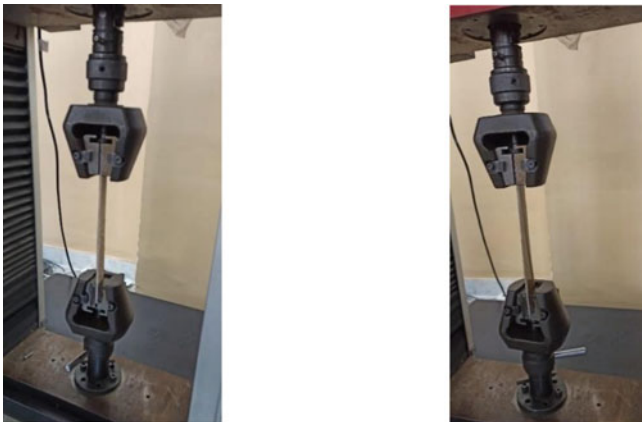
(a) Hemp-linen/epoxy reinforced biocomposites under tensile strength testing (b) Hemp-epoxy biocomposites under tensile strength testing
