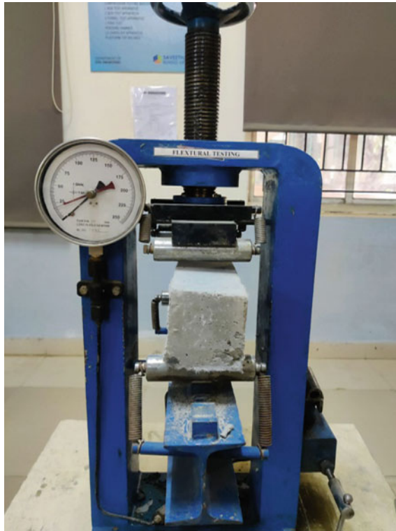
Fig. 4 Manually handled flexural testing machine at the time of sampling testing which was used for the study
