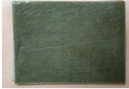
Fig. 4 Hemp-linen hybrid and epoxy-reinforced biocomposites
