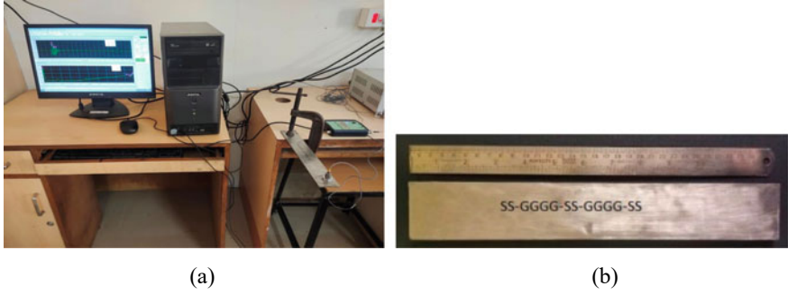
Fig. 2 a Test setup for modal analysis of cantilever beam using FFT analyzer, b Cantilever beam test specimen used for modal analysis
