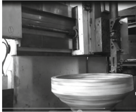
Fig. 5 Cone liner pattern manufacturing at CNC VTL machine
