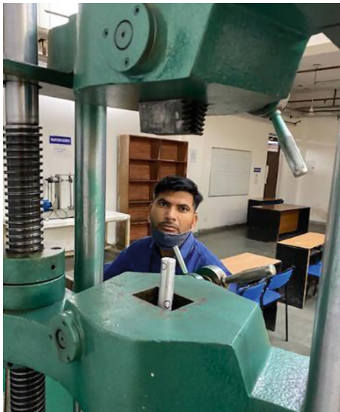
Fig. 6 Conducting tensile strength test on UTM
