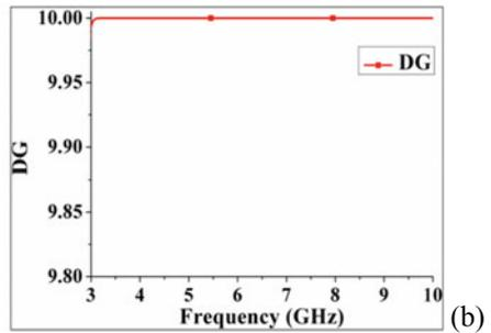
Fig. 5 Simulated **a** envelop correlation coefficient, **b** diversity gain of the proposed antenna
