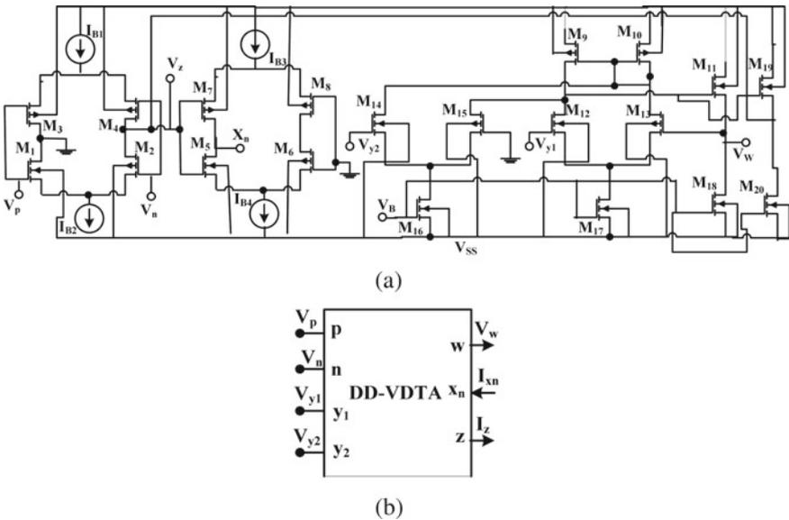
Fig. 1 DD-VDTA a CMOS structure b block diagram
