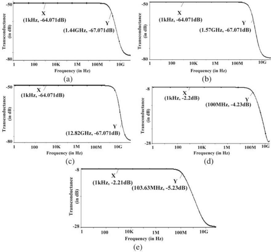
**Fig. 4** AC characteristics of DD-VDTA **a** frequency response of  $g_m$  from port  $z$  to  $v_p$  **b** frequency response of  $g_m$  from port  $z$  to  $v_n$  **c** frequency response of  $g_m$  from  $z$  to  $v_x$  **d** frequency response of  $V_{y1}/V_w$  **e** frequency response of  $V_{y2}/V_w$
