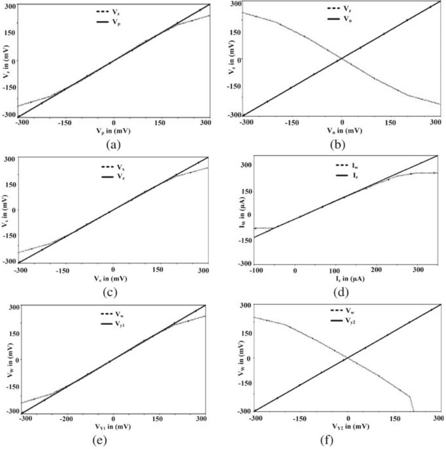
**Fig. 3** DC voltage variation behaviour of DD-VDTA at different port **a** voltage  $z$  to **p** **b** voltage  $z$  to **n** **c** voltage  $x$  to  $z$  **d** current  $w$  to  $z$  **e** voltage  $w$  to  $y_1$  **f** voltage  $w$  to  $y_2$
