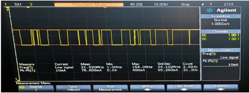
Fig. 8 The envisioned TRNG’s output waveform is constructed upon ADPLL and LFSR (15-LFSR)
