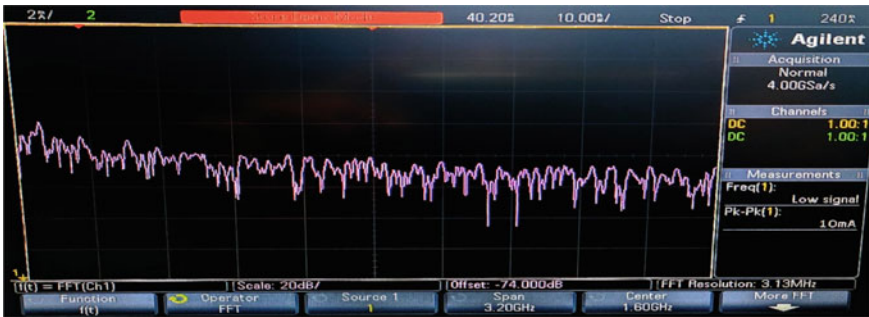
Fig. 9 FFT output waveform of TRNG build on ADPLL along with LFSR (15-LFSR) architecture
