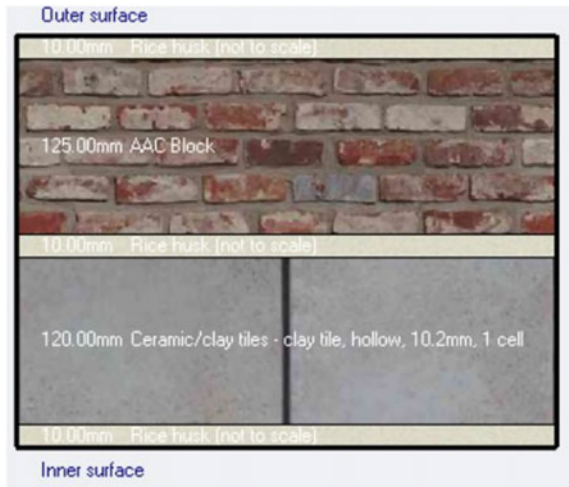
Fig. 1 Structural details of insulation system (Wall)
