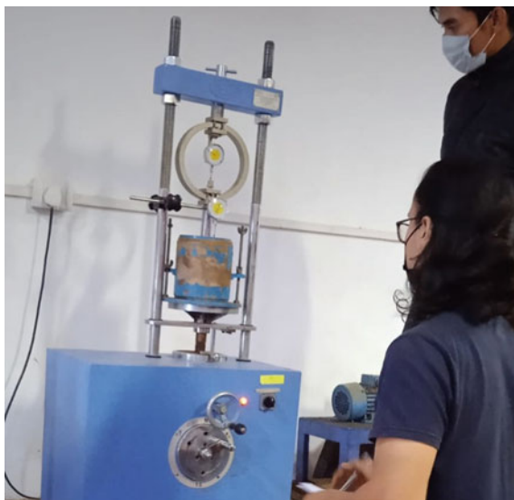
Fig. 3 CBR testing of soil samples
