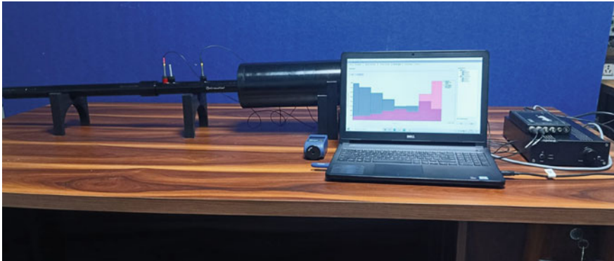
Fig. 2 Sound impedance tube for measurement of sound absorption characteristics in higher frequency range
