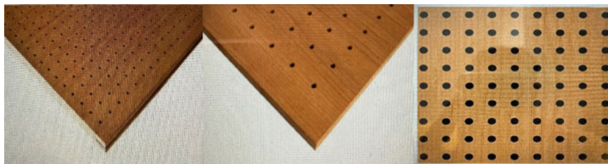
Fig. 1 The perforated panels with different specific hole diameters a d = 2 mm and P = 2.2\% b d = 6 mm and P = 4.4\% c d = 9 mm and P = 6\%
