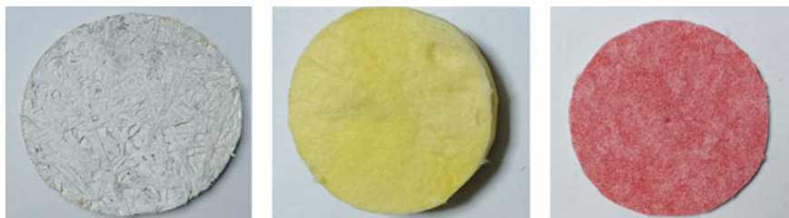
Fig. 3 Pine wood board, glasswool and PET acoustic panel (100 mm diameter)
