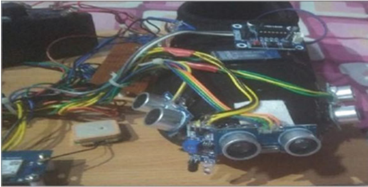
Fig. 9.1 Integrating ultrasonic sensors, IR sensor to the toe cap and Bluetooth and Voice module on the vamp of the shoe
