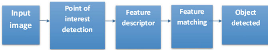
Fig. 12.2 Flow chart of SURF algorithm
