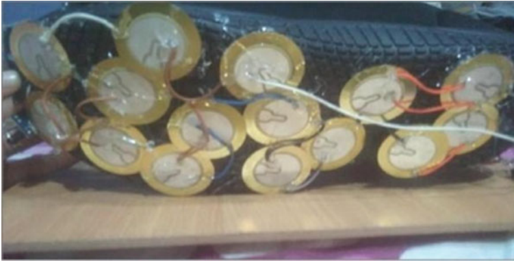
Fig. 9.3 Piezoelectric plates lined up on the sole of the shoe
