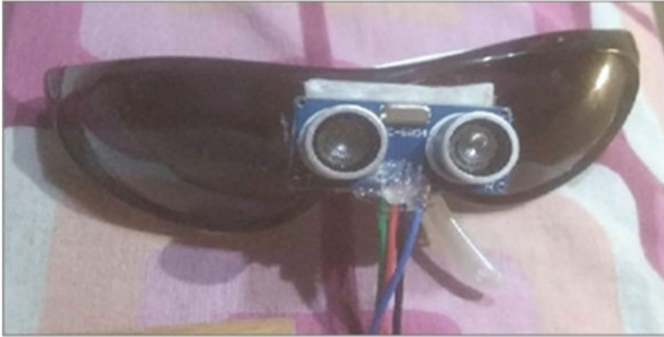
Fig. 9.5 Image of HC-SR04 sensor fixed on the bridge of the glass
