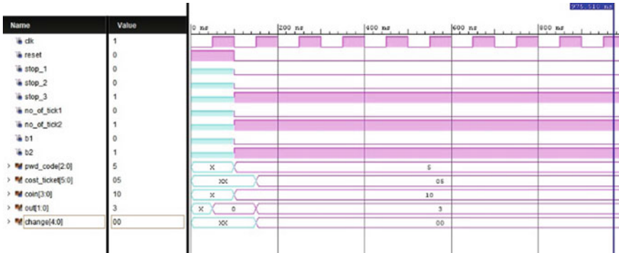
Fig. 4 I/O waveform simulation with rebate condition
