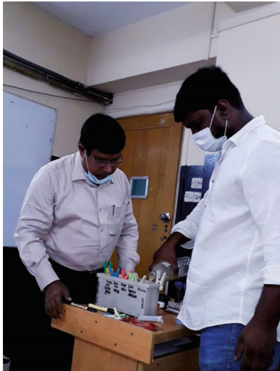
Fig. 2 Ginger, pumpkin, balsam, potato, jute leaves, and onion extracts are put into the 6 compartments as an electrolytes
