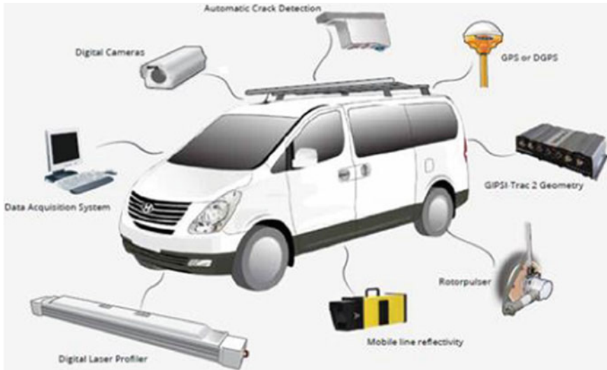
Fig. 3 Components of Integrated Survey Vehicle [3]
