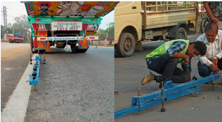
Fig. 6 Collection field deflection data using BBD test -static method
