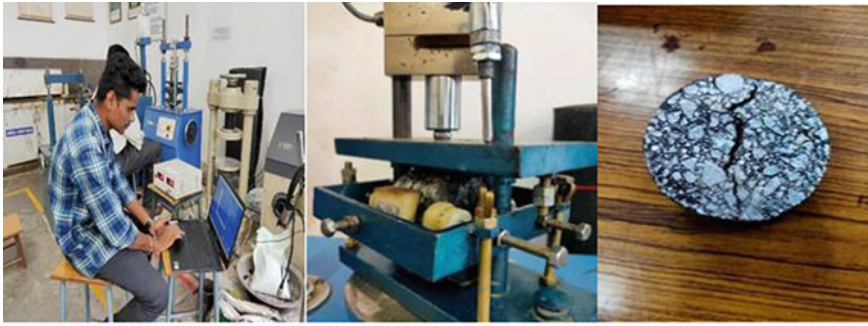
(a) In-direct tensile test process (b) In-direct tensile test process (c) field sample
