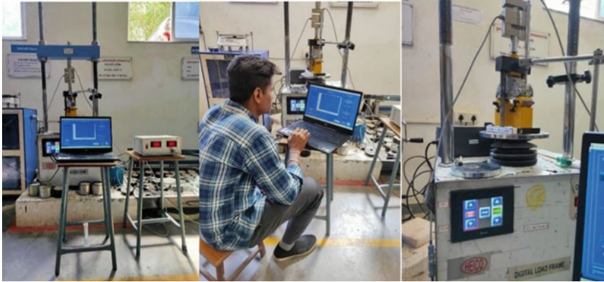
Fig. 11 Fracture properties conducted through semi-circular bending test
