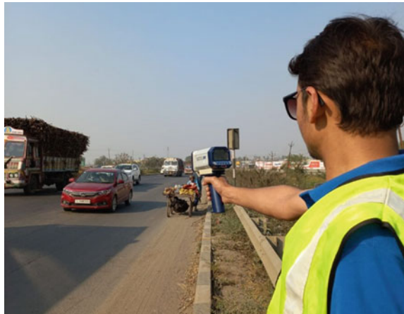
Fig. 4 Spot speed data collection through radar gun
