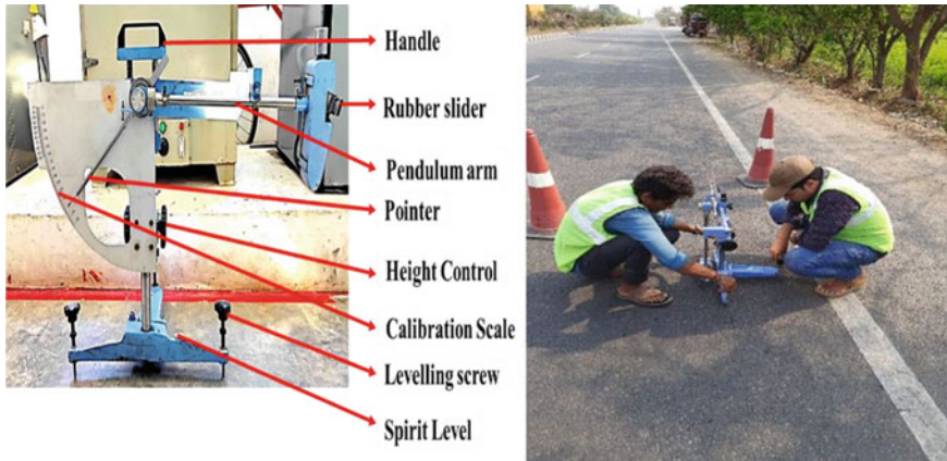
Fig. 4 Skid resistance test conducted on study locations
