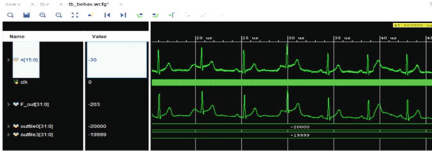
Fig. 7 Denoised ECG signal on Xilinx Vivado 2018 platform
