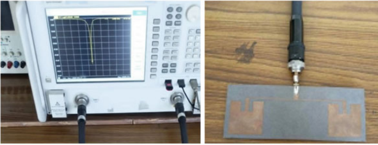
Fig. 2 S_{11} Measurement of developed antenna on vector network analyzer
