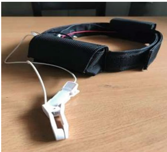
Fig. 1 Prototype headband with Neurosky TGAMI (EEG sensor)
