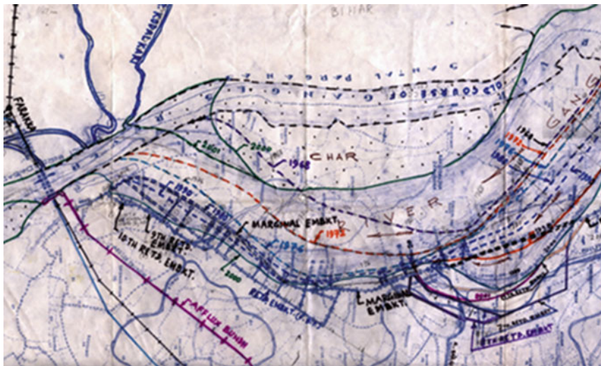
Fig. 5 Retired embankments to close the breach of embankment near Manikchak
