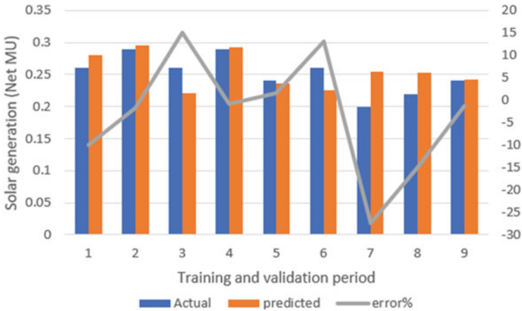
Fig. 7 Error percentage curve between the actual and the predicted solar generation in (net Mu) using 7-day data period interval
