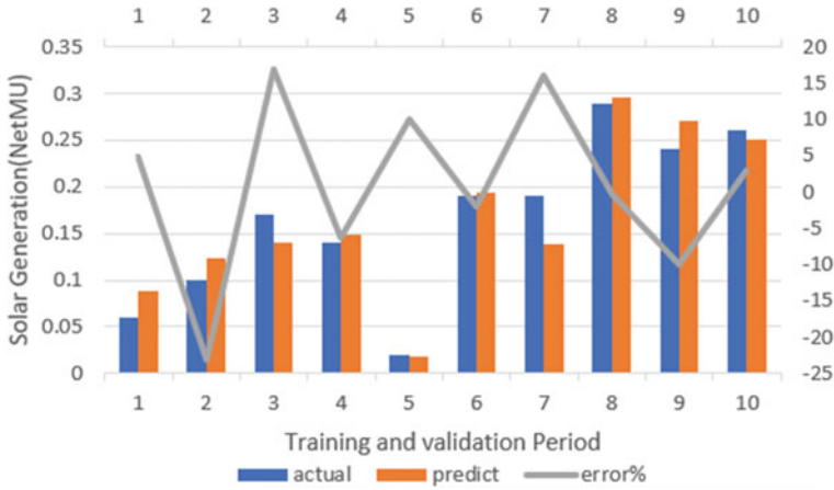
Fig. 6 Error percentage curve between the actual and the predicted solar generation in (net MU) using 15-day data period interval
