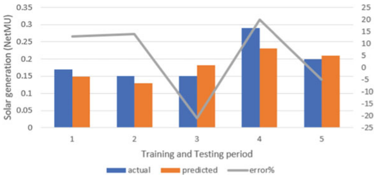
Fig. 5 Error percentage curve between the actual and the predicted solar generation in (net MU)
