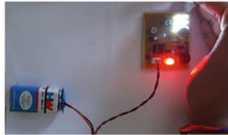
C Circuit with low intensity of surroundings light. (when low intensity of surrounding light is sensed by LDR the device increases its intensity)
