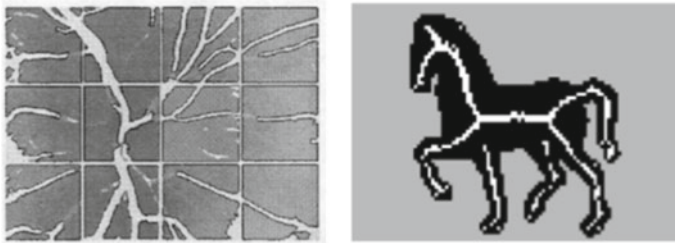
Fig. 1.8 Examples of image contour and skeleton extraction using SCAMP PPA. Left: Extracted Retinal Vascular Tree, Figure from [50]. Right: Extracted skeletons, Figure from [47]
