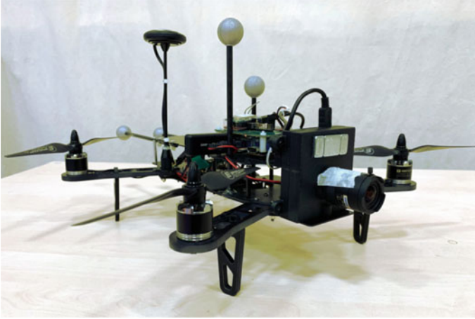
Fig. 1.10 Quadrotor setup for the drone racing with a front-facing SCAMP (Figure from [74])
