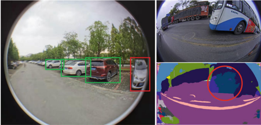
Fig. 2.2 False results caused by the distortion of the fish-eye image. The red bounding box represents false negative detection results, and the area in the red circle represents false positive segmentation results
