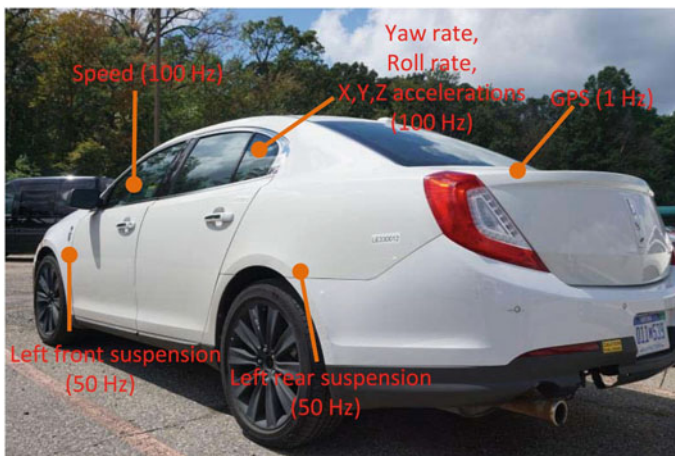
Fig. 11.4 In-vehicle sensors for vibration signals collection [27]
