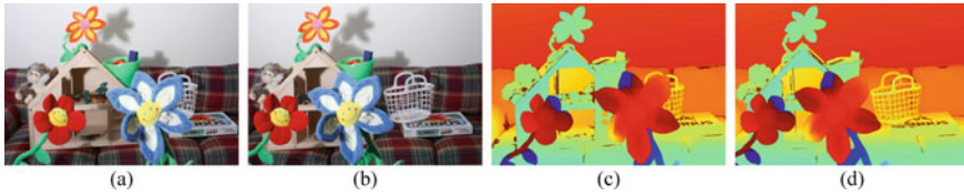
Fig. 3.5 a Left stereo image; b right stereo image; c left disparity map; d right disparity map
