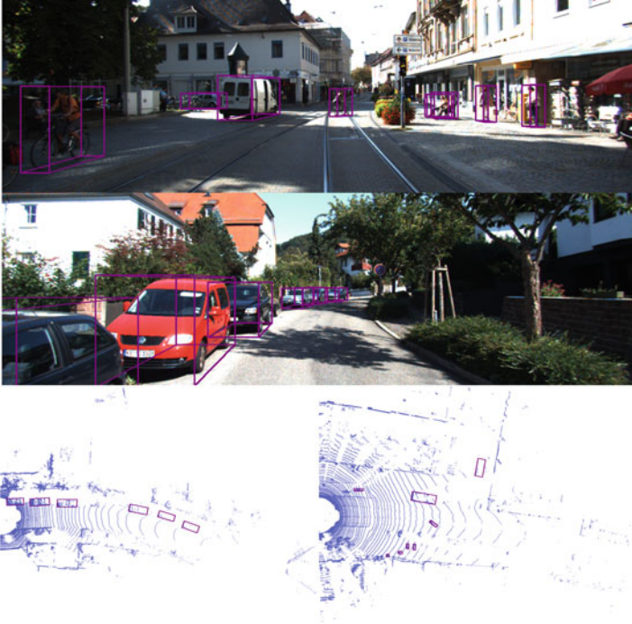
Fig. 5.3 Visualization rendered from the KITTI 3D object detection dataset [20]. The bottom row contains the BEV images of the two scenes in the upper rows
