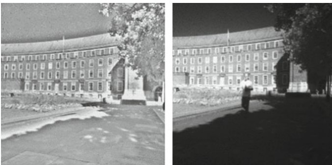
Fig. 1.6 Examples of two images with(left)/without(right) HDR algorithms towards the same scene in an outdoor environment
