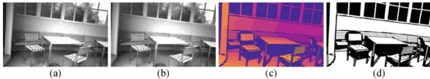
Fig. 3.19 Example images of eth3d benchmark [16]. a Left stereo image; b right stereo image; c ground truth disparity map; d noc mask
