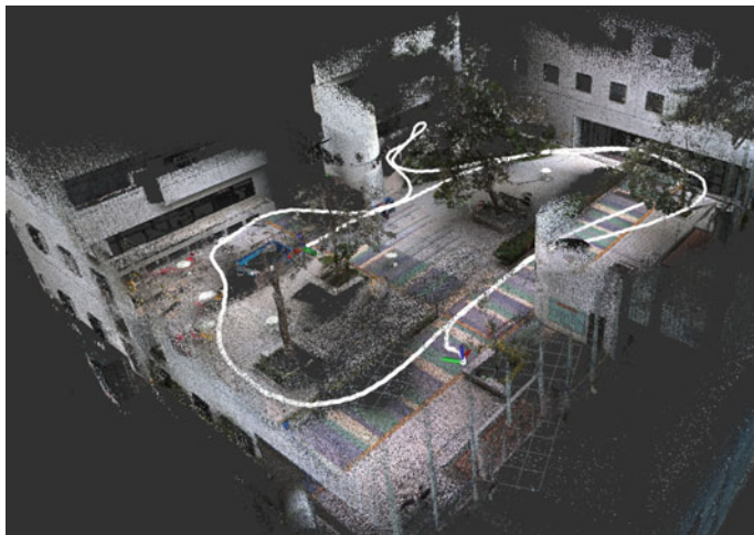
Fig. 7.17 R3LIVE’s results: estimated trajectory (white) and colored point cloud
