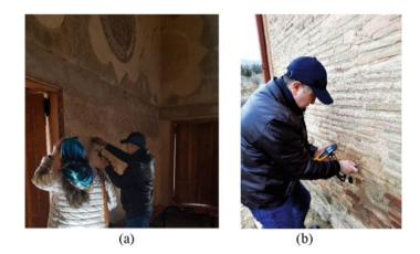
Fig. 6 Field measurements of temperature and humidity on the internal **a** and enclosures' external surfaces **b**
