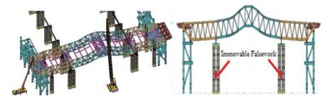
Fig. 2 Construction diagram of "cumulative sliding of structure"
