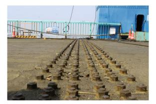
of the bolt is calculated according to the regression equation. During the test, the clamping force of the test bolt after final tightening (hereinafter referred to as "initial clamping force") is more than the design value of M20 high-strength bolt clamping force (155kN), which is about 1.1 times of the design value of clamping force.
