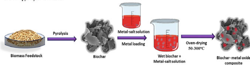
Fig. 12.5 Schematic representation of pre- and post-pyrolysis treatment used for modification of BCs
