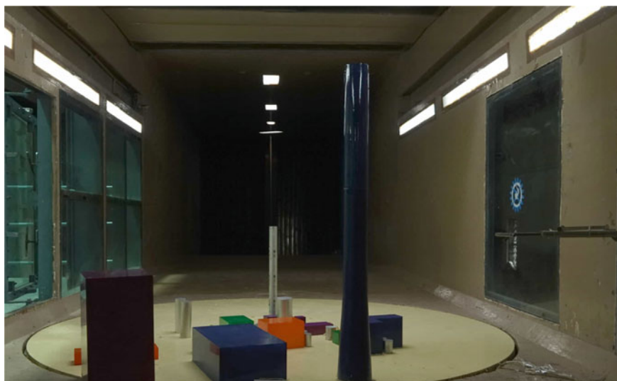
Fig. 2 Wind tunnel setup for interference case-2 showing the principal chimney with the interfering chimney and surrounding building structures for 345^\circ angle of wind incidence
