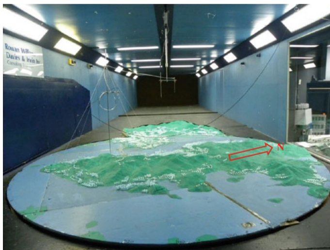
Fig. 7 1:3000 scale topography model
