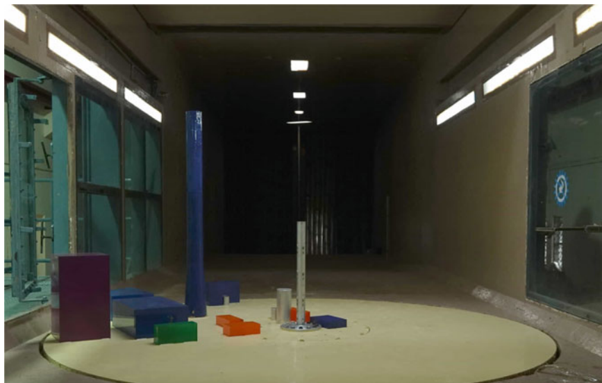
Fig. 1 Wind tunnel setup for interference case-1 showing the principal chimney with the interfering chimney and surrounding building structures for 120^\circ angle of wind incidence
