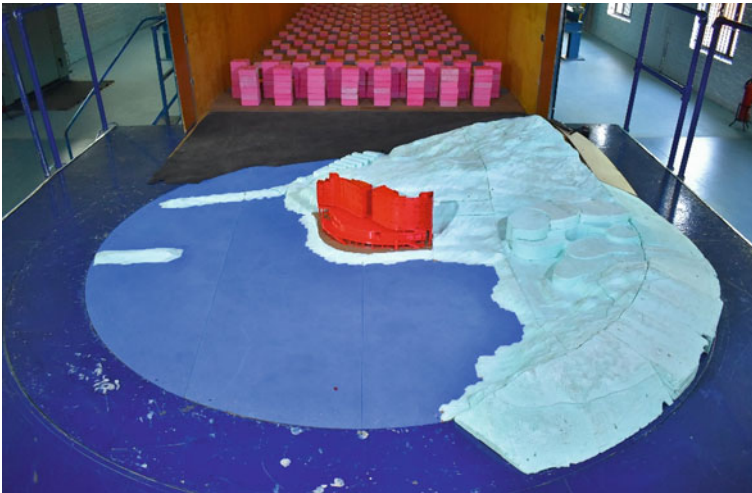
Fig. 3 Wind tunnel test at 1:300 scale
