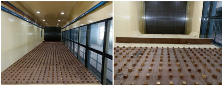
Fig. 1 Experimental setup for terrain simulation studies
