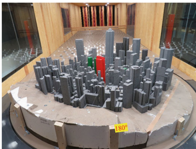
Fig. 8 Wind tunnel test at a large scale of 1:300
