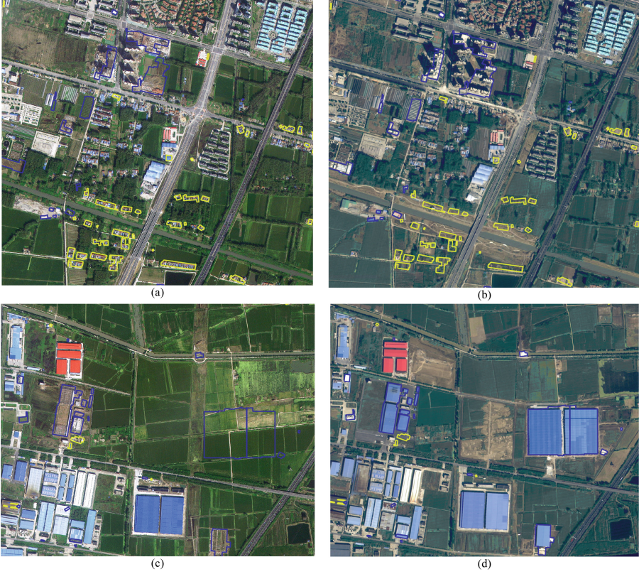
Fig. 4. Detailed building semantic change comparison. (The blue color and yellow color are building increase, building decrease, respectively). (a) and (c) is the former time-phase image, (b) and (d) is the latter time-phase image.
